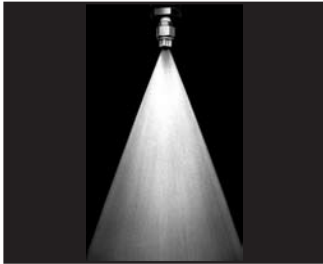
Thin rectangular pattern produces medium-sized drops.
