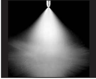
Low capacity spray producing small drops in a hollow cone pattern.
