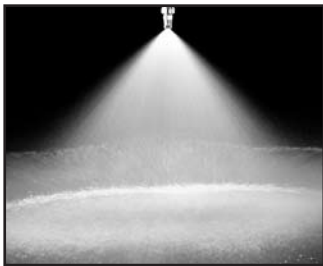
Uniform, round and full spray pattern with medium-to-large sized drops.
