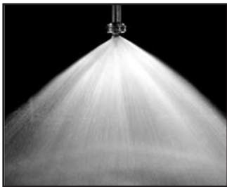
Full cone pattern with relatively coarser drops.
