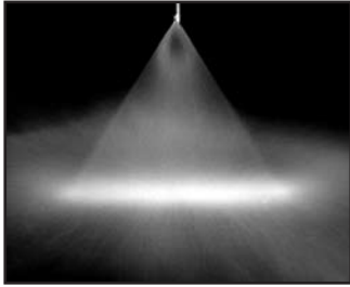
Tapered edge flat spray pattern with medium-sized drops.
