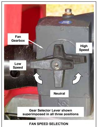
The neutral position of the gearbox enables the pump and agitators to be operated without the fan. This position can be used when running the sprayer to mix the chemical solution.
