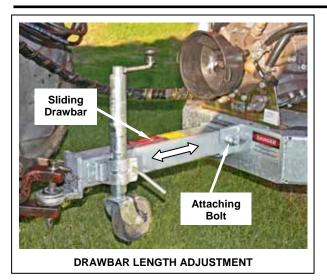
Securely tighten the attaching bolt. Raise the sprayer with the jack to remove the support stand and connect to the tractor as previously described.
