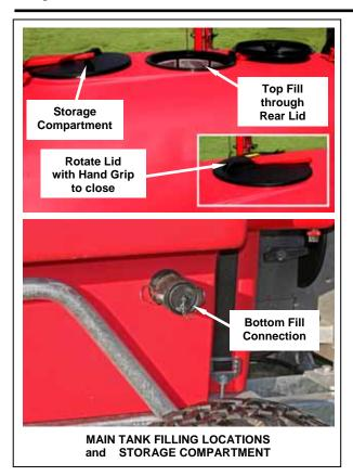
Filling the Main Tank using Bottom Connection The main tank can be filled through either the top or bottom but the recommended method is through the bottom fill connection, which is more convenient and prevents chemicals frothing. It is also safer as the tank can be filled from ground level.
