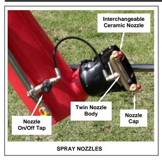
Spray output at a particular pressure can be varied by fitting nozzles with different size orifice plates. The nozzles are colour coded to assist identification. Refer to the Nozzle Chart in the Calibration section.
