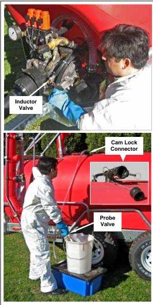
CHEMICAL PROBE Always wear the protective clothing recommended by the chemical manufacturer.
