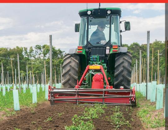
Silvan's Brevi range provides various features to help you choose a power harrow tailored to your needs. These features include phased rotors, Superfast quick-release blade options, adjustable hitches, hydraulic folding, robust gearboxes, and gear drives.
